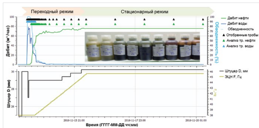
Рис. 5 — Отбор проб и замеры во время исследования скважины X31 в ноябре 2016 Fig. 5 — Sampling and measurements during production logging in well X31 in November, 2016
